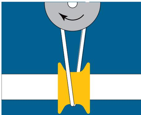
**Quiet** The elastomeric belt holds the rollers and the drive bushings firmly under tension. This eliminates the conventional rattling, jiggling and jangling.... fewer moving parts make less noise
