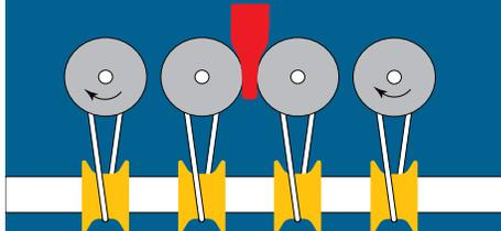
**Sensible** Each roller, drive bushing and belt operate like a slip clutch... the torque to each roller is adequate to drive the roller, but the slip clutch effect allows each roller to stop.
