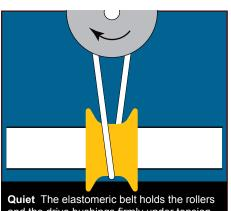
**Quiet** The elastomeric belt holds the rollers and the drive bushings firmly under tension. This eliminates the conventional rattling, jiggling and jangling.... fewer moving parts make less noise
