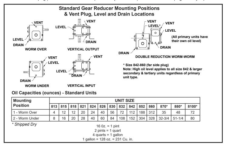
3. CLEANING - After approximately two to three weeks of operation the reducer MUST be drained, flushed out, and refilled to the proper level with fresh oil. (This is done to remove brass particles caused during the normal wear-in period of the worm gear.) Afterwards, the oil should be changed in your reducer every 2500 hours or every 6 months, which ever occurs first.
