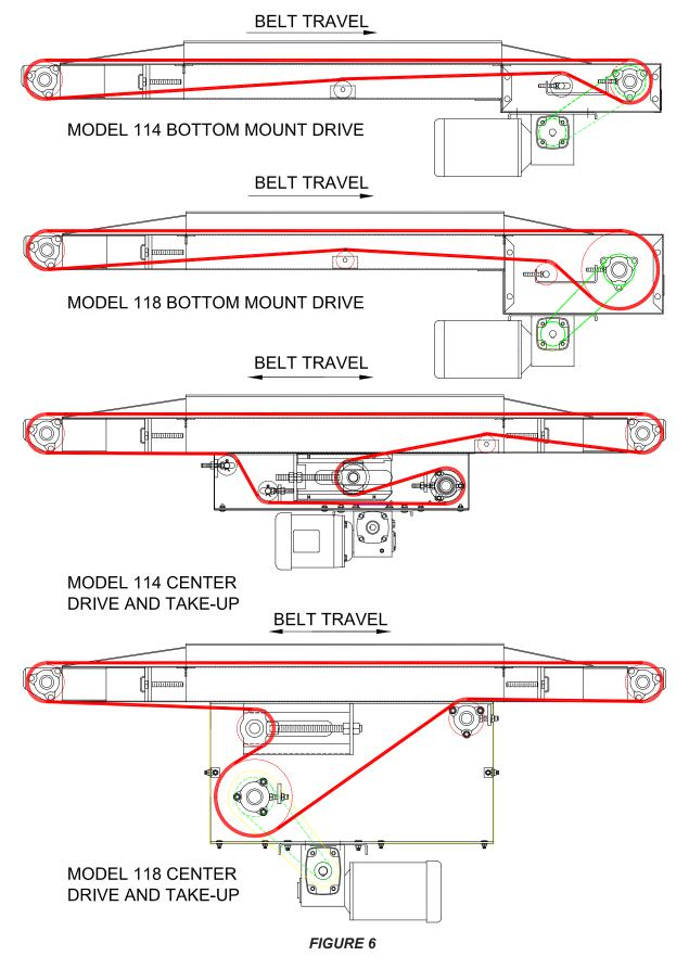
4. After making sure the conveyor is cleared off and the drive pulley is moving the belt in the correct direction, run the conveyor. Take up slack belt with the take-up provided until there is no slippage between the drive pulley and the belt.
