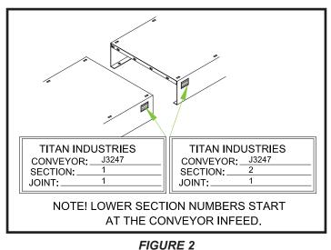
2. Layout a line on the floor to represent the centerline of the conveyor. As frame sections are bolted together make sure the frame remains centered on the line.
