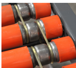
Urethane O-Belt Driven Roller
