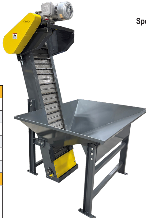
Custom hopper for delicate parts
