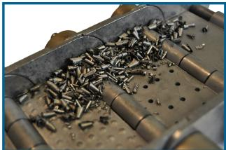
2-1/2" RADIAL SIDEWINGS Exclusive Titan radial sidewing prevents jamming, even with the smallest chips & fines.
