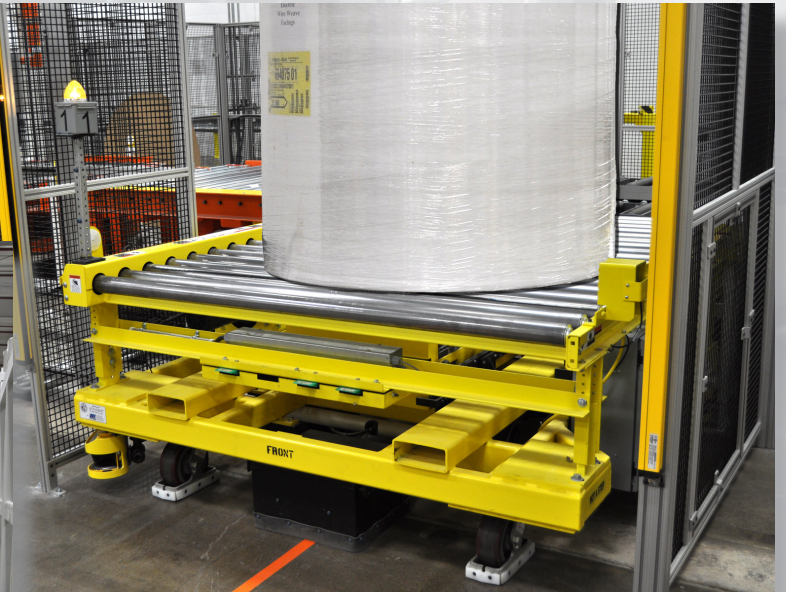
A Titan Designed Automated Guide Vehicle for a major consumer product manufacturer carrying rolls of plastic from workstation to warehouse.
