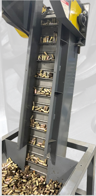
Shell Casings loaded on belt from hopper
