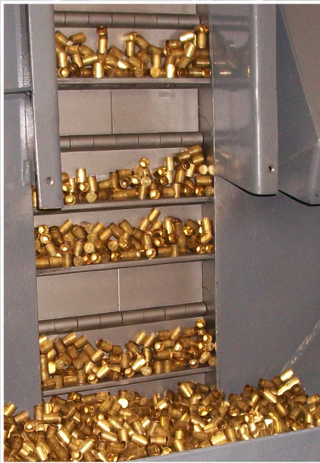
Shell Casings loaded on belt from hopper
