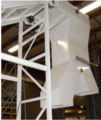
Special delivery chute for bulk material
