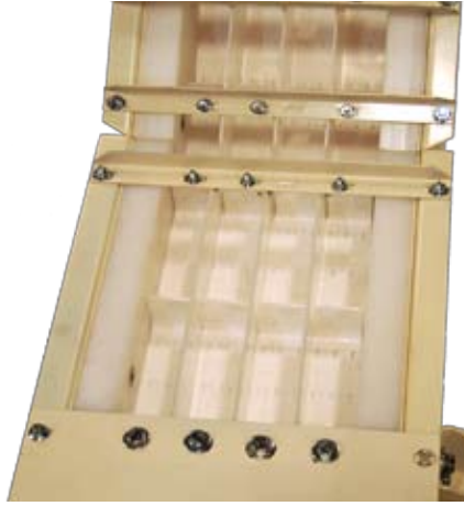
Titan designed and built plastic belt conveyor with 4 lanes for transporting colored plastic pellets to packaging
