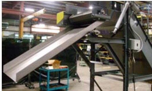
Special pneumatic chute for diverting material to specialized bins.
