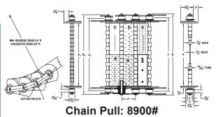
Belt Styles: 1-Plain, 2-Perforated, 3-Double Perforated 4-Pimpled, 5-Pimpled & Perforated, 6- Impact Bar
