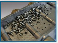
**Exclusive Titan radial sidewings** eliminate the gaps that cause parts damage and material seepage.
