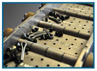
Titan hinged steel belt was developed to handle stampings, metal scrap, paper scrap, chips, turnings, castings and parts, plus numerous other materials. The standard 2 1/2" pitch belt is interchangeable with other conveyor or belt manufacturers. All parts on standard belts are available from stock. Standard profile and low profile sidewings are available. Belt widths from 4" to 48" in increments of 2".
