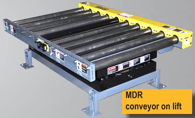
MDR conveyor with special siderails to shift product
