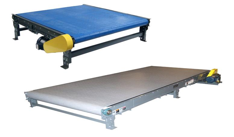
Titan's **Pallet Pro Heavy Duty Plastic Belt Conveyor** solves the problem of conveying and transferring pallets that are irregular, imperfect or peg type pallets better than standard roller type conveyors. The heavy duty plastic belt enables end or side loading, allows for minimum transfer gaps and is bi-directional. Industries such as automotive, paper, corrugated, distribution, bottling, cardboard and others will benefit from this innovative design.
