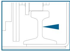
H.D. 25# rail track reduces wear factors and improves conveyor integrity.
