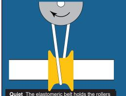
**Quiet** The elastomeric belt holds the rollers and the drive bushings firmly under tension. This eliminates the conventional rattling, jiggling and jangling.... fewer moving parts make less noise
