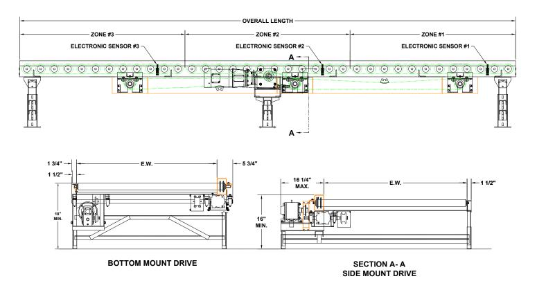
A Chain Driven Live Roller Conveyor is set up with individually controlled "zones" by installing electronic sensors at equal intervals along the conveyor. Power to individual zones comes from a main chain drive that runs the length of the conveyor. Each zone is driven off the main drive and activated or deactivated with an air operated clutch controlled by an electronic sensor.
